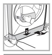
1. Take off the cover panel on the front of the machine by first pressing it in the centre and then pushing downwards on both sides until you can remove it (see figures).
